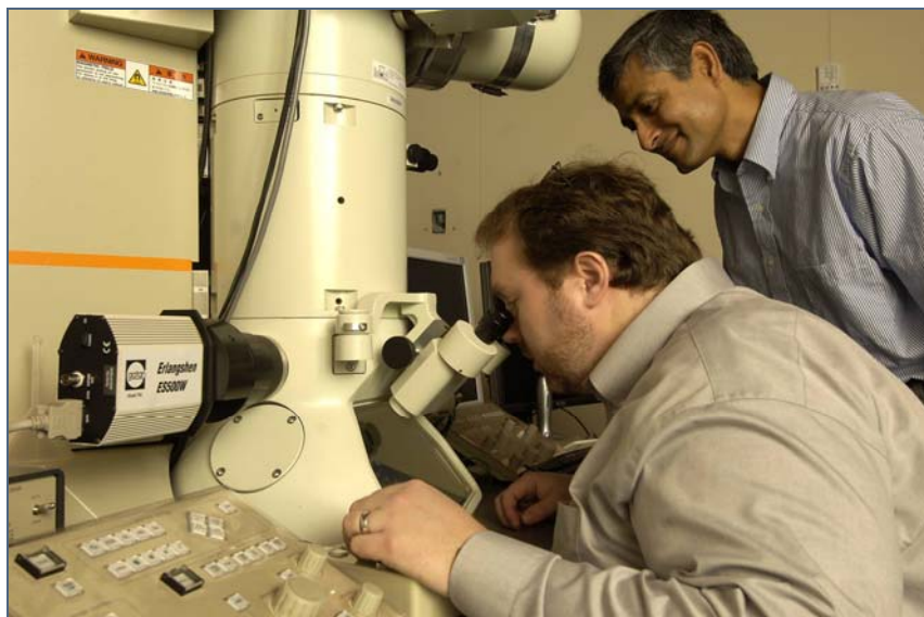
Drs. Soumitra Ghoshroy and Douglas Blom of the Nanostructures CoEE use the JEOL 2100F aberration-corrected STEM to study the composition and structure of nanomaterials in USC's Electron Microscopy Center.
