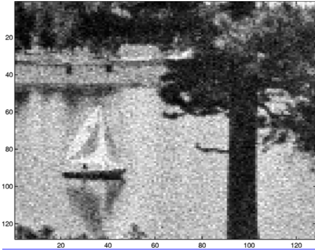
Fig. 5. Local ML estimate using photon-correlated beams. The photon correlation parameter \beta is 0.01. The remaining parameters are the same as those in Fig. 4.
