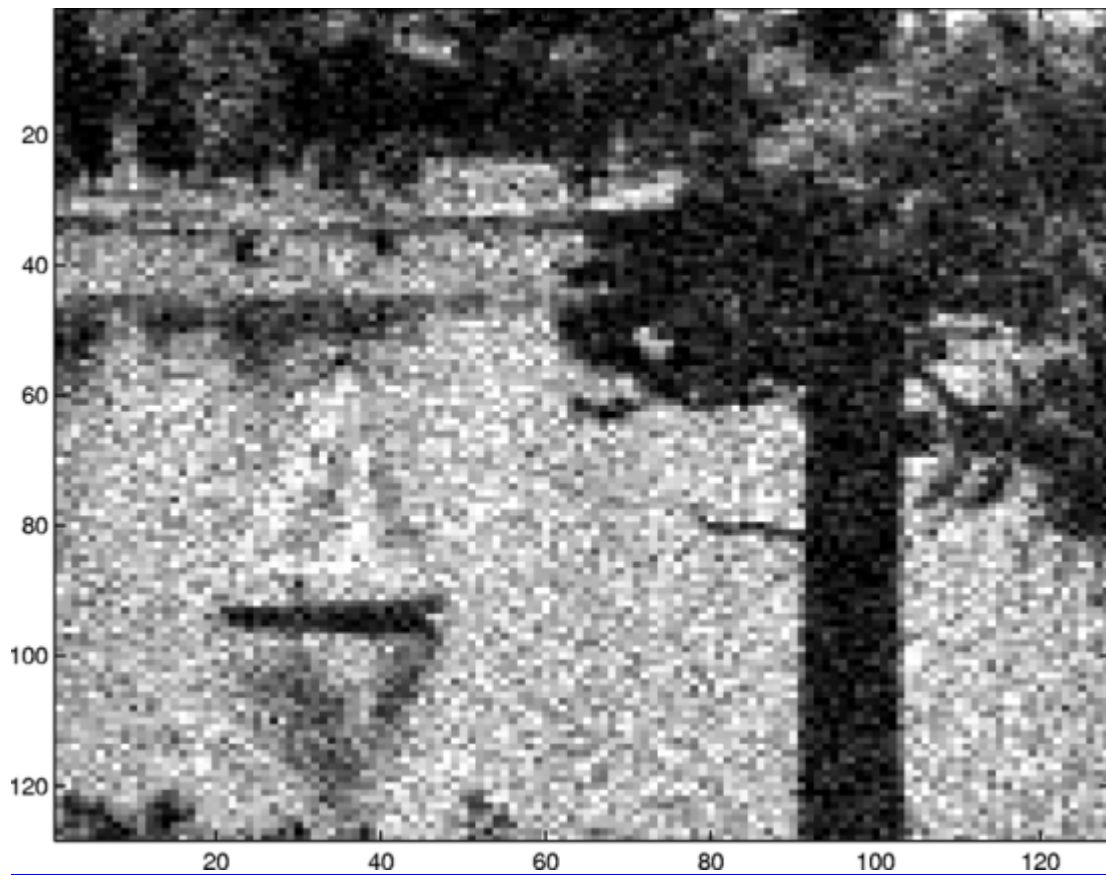
Fig. 8. Conventional ML estimate in the presence of background noise and under conditions of nonideal detection. The background-noise parameter nb and the signal parameter np are 5 and 50, respectively. The detector quantum efficiency \eta is 0.8.
