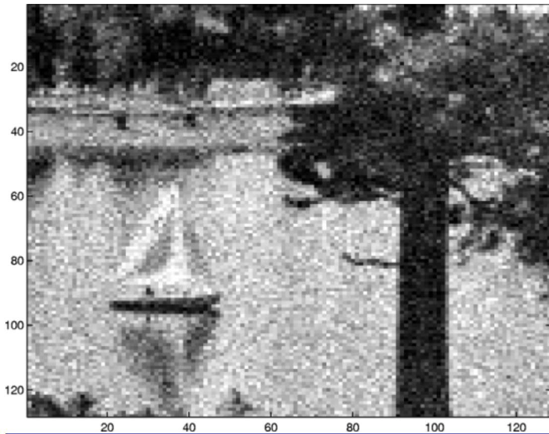
Fig. 7. Local ML estimate using photon-correlated beams in the presence of background noise when the photon correlation parameter \theta is 0.01. The remaining parameters are the same as those in Fig. 6.
