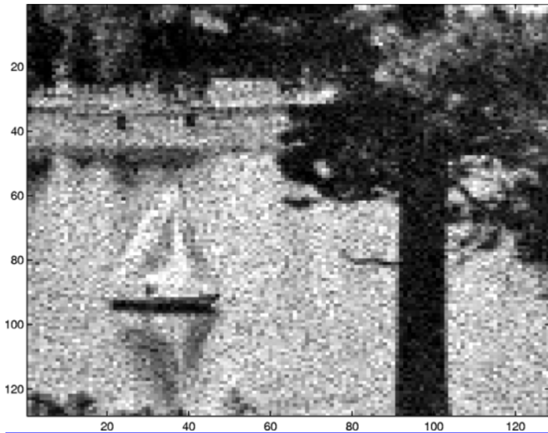
Fig. 4. ML estimate of the true image using the conventional setup. Ideal conditions of background noise ( nb=0 ) and quantum efficiency ( \eta=1 ) are assumed. The signal parameter np is 50.
