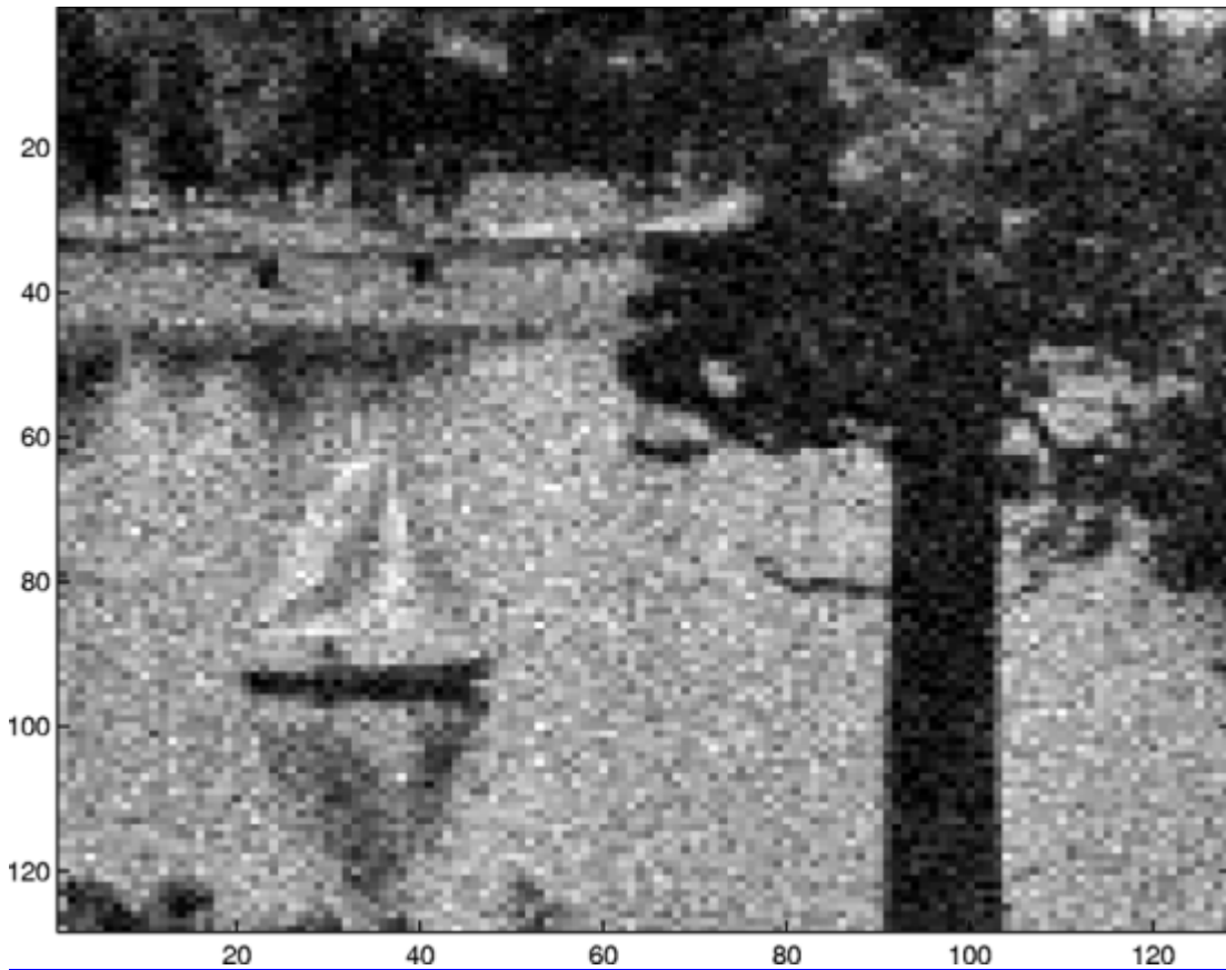
Fig. 9. The local ML estimate using photon-correlated beams in the presence of background noise and under conditions of nonideal detection. The photon correlation parameter \beta is 0.01. The remaining parameters are the same as those in Fig. 8.
