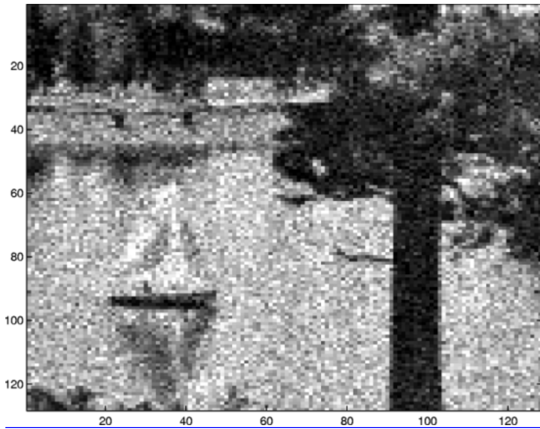
Fig. 6. Conventional ML estimate in the presence of background noise under ideal detection conditions ( \eta=1 ). The background-noise parameter nb is five and the signal parameter np is 50.
