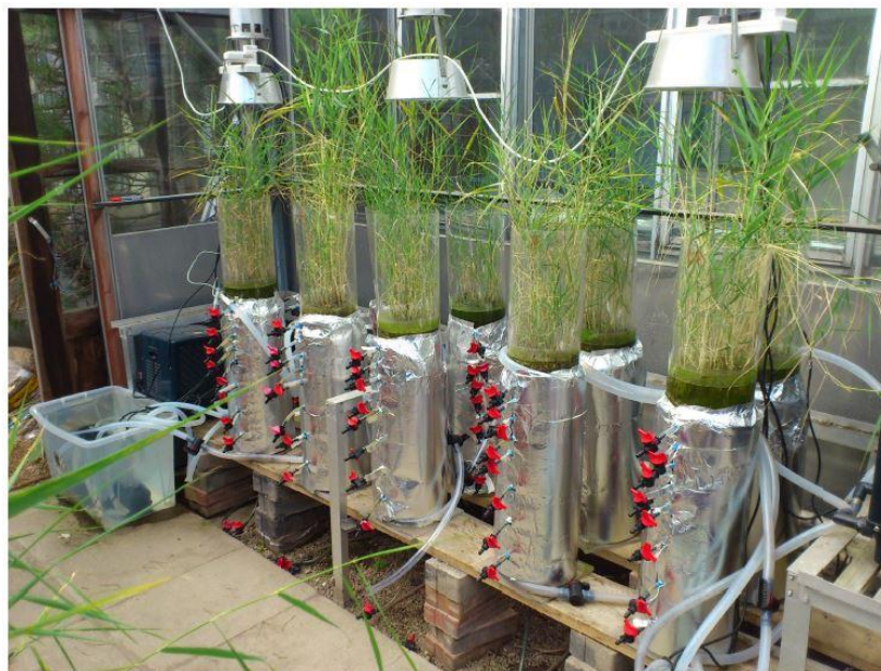
Figure 1.6 Phytoremediation process for removal of inorganic contaminants. (Graphic Courtesy: National Institute for Biotechnology and Genetic Engineering)
