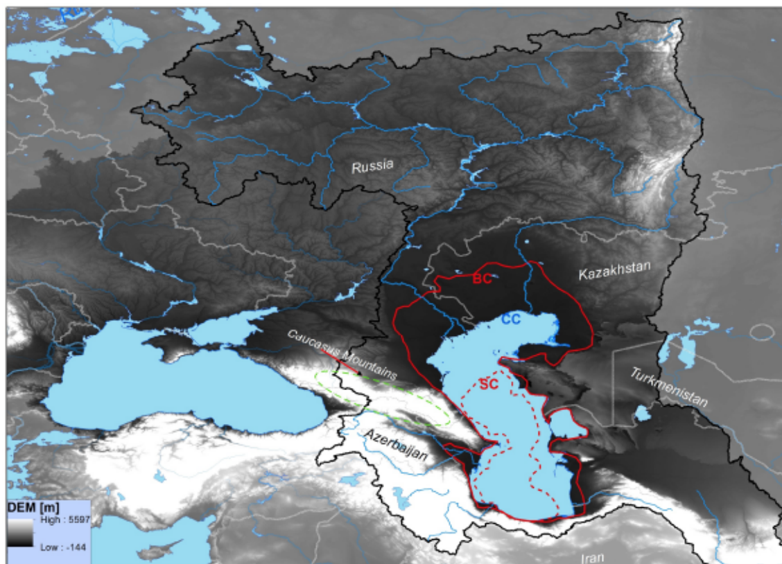
Figure 5.1: Study Area. High resolution DEM contours of Caspian Sea surface areas (shown by red solid line (big Caspian-BC), red broken line (small Caspian-SC) and light blue area (current Caspian-CC)). The catchment area is depicted by black solid line. Blue and grey solid lines represent rivers and country borders respectively. Elevation change is shown by colour shades of white-grey-black.
