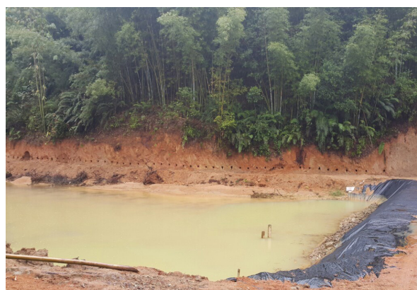
FIGURE 2 In situ leaching pond for ion-adsorption clay REE deposit, China. A low technology technique is used whereby drainage holes at the rear of the collection pond bring the leach solution down the hillside through the weathered granite. In theory, this could be a low environmental impact method to produce REEs, but it depends on the chemicals used and how well they are controlled. PHOTO COURTESY OF ALAIN ROLLAT.
