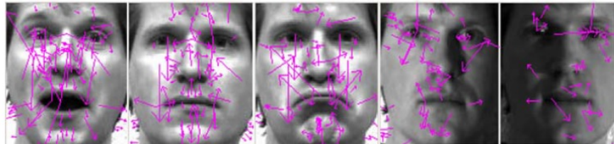
Figure 2.5: An example of images with extracted SIFT features. The images represent the same object with different expressions and illumination (Zhang et al., 2008)
