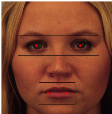
Figure 4.1: Four points detection(the two eyes centres and two point on the mouth).
