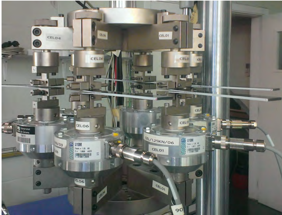
Fig. 2.12.: Multi-fatigue test device with 6 specimens.
