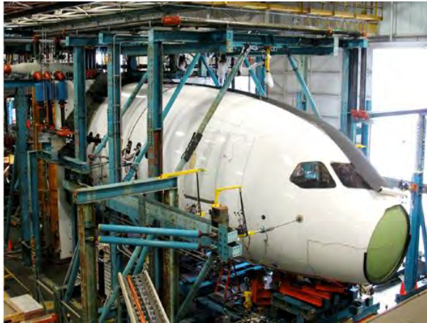
Fig. 1.1.: Full-scale fatigue test on Boeing 787 [39].
