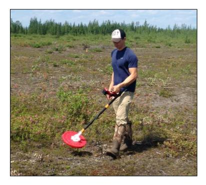
Figure 3.10: KT-20 3F S/C meter operated by field assistant Dillon Montague.
