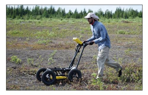
Figure 3.11: Sensors and Software GPR Noggins SmartCart system in the field.
