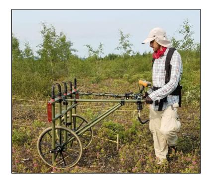
Figure 3.8: The author with the Sensys MXPDA magnetometer cart.
