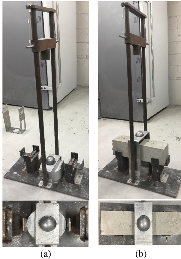
Figure 3-7 Impact tests (a) drop-weight test (ACI-544), (b) flexural loading test
