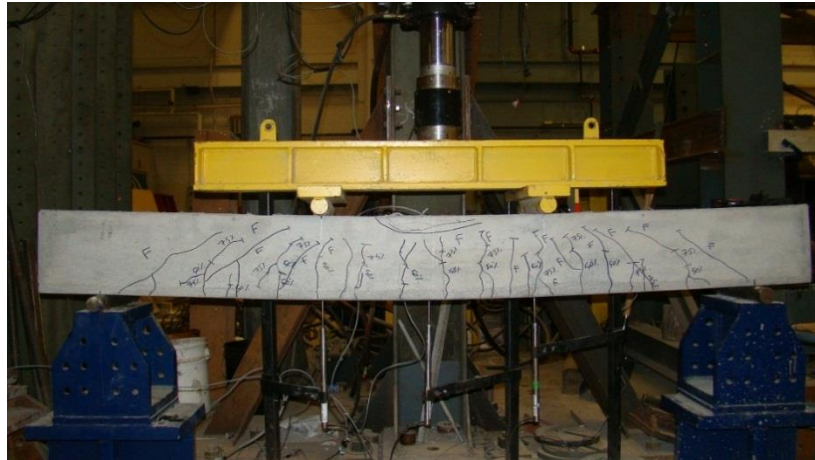
Figure 3-9 Typical test setup, dimensions, reinforcement, and failure mode of tested beams in flexure
