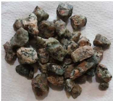
Crushed stone (coarse aggregate)
