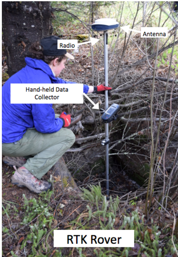
Appendix 1: Photo 15- This is the RTK rover with a secondary antenna on top of the rod and the data collector part way
