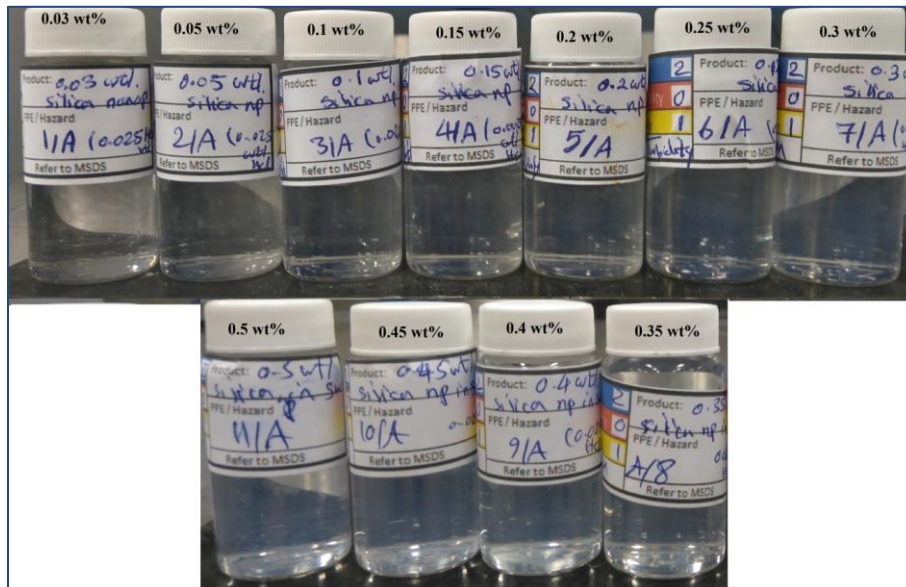
Figure 3-12: The visual status of silica nanoparticles with different concentrations (the concentrations are written on the top of each sample) in the solution of seawater with 0.025 wt% HCl after 48 hours.
