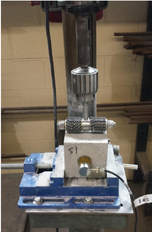
Figure 3-1 Abrasion Test Set up with AE monitor
