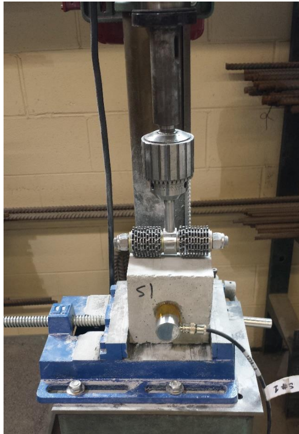
Figure 4-1 AE and Abrasion Test Setup
