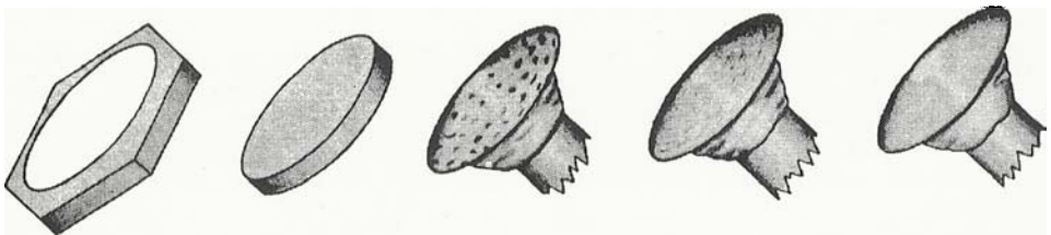
FIG. 5. Cabochons at various stages of cutting and polishing. Left to right: trimmed from slab; ground to outline; after rough grinding; after sanding; polished.
