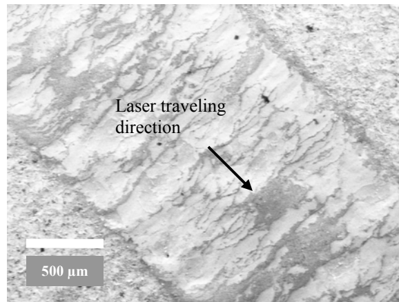
Figure 7. SEM image of a CO 2 laser polished track that has undergone Surface Over Melt, 50x. Adapted from Reference 6.
