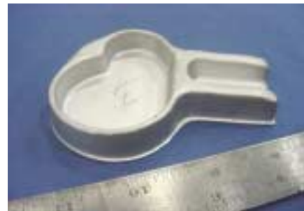
Fig. 3 Part used for initial trial of the die
