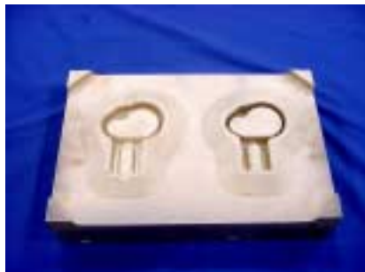
Fig. 2 Die made from Prometal technique
