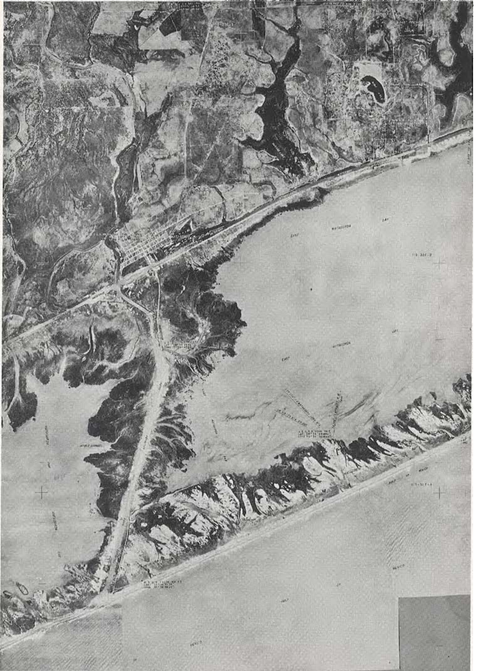
FIG. 1. Colorado River delta with offshore bar (barrier island) in foreground; scale 1" = 6,000'. Deltas form and grow seaward at the mouths of rivers at places where the strength of wave and ocean currents exceeds that of the stream currents. Waves and ocean currents continually rework the deposits and reshape the delta margins. (Photograph by Edgar Tobin Aerial Surveys, San Antonio, Texas.)
