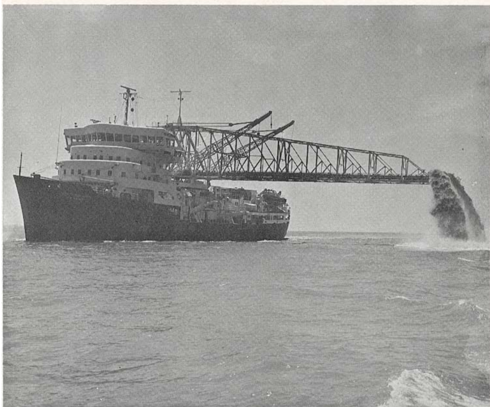
FIG. 5. U. S. Army Corps of Engineers hopper dredge "McFarland" during a dredging operation. Sand, gravel, mud, oyster shell, and other debris are sucked from the channel through an intake pipe and spilled to a side of the channel through the spoil pipe supported along the boom. (Photograph by Corps of Engineers, U. S. Army, Galveston District, Galveston, Texas.)
