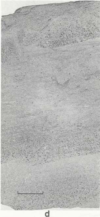
figure 15 (con.) (d) Burrows within single coset; 6,552 m (21,492 ft). Scale bars in b, c, and d equal 2 cm; core from Pan American No. 1A Alamo National Bank.
