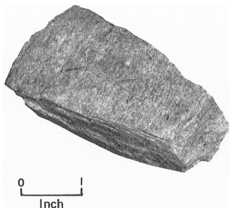
Feldspar cleavage fragment from Llano County, Texas. The two directions of good cleavage meet at an angle of about 90°.
