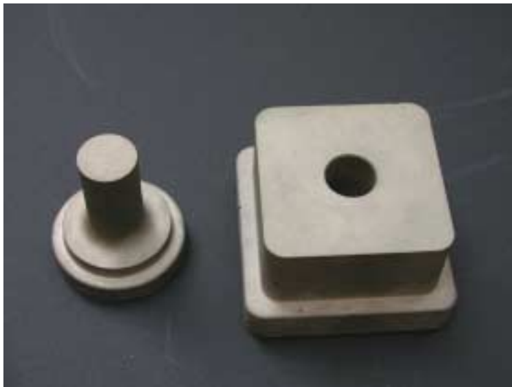
Figure 1: SLS® core and cavity insert made with LaserForm™ ST-100.
