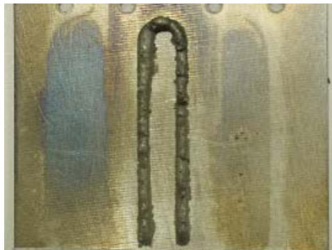
Figure 15. Single-layer U-shape deposit SLM laid using an open loop control scheme.
