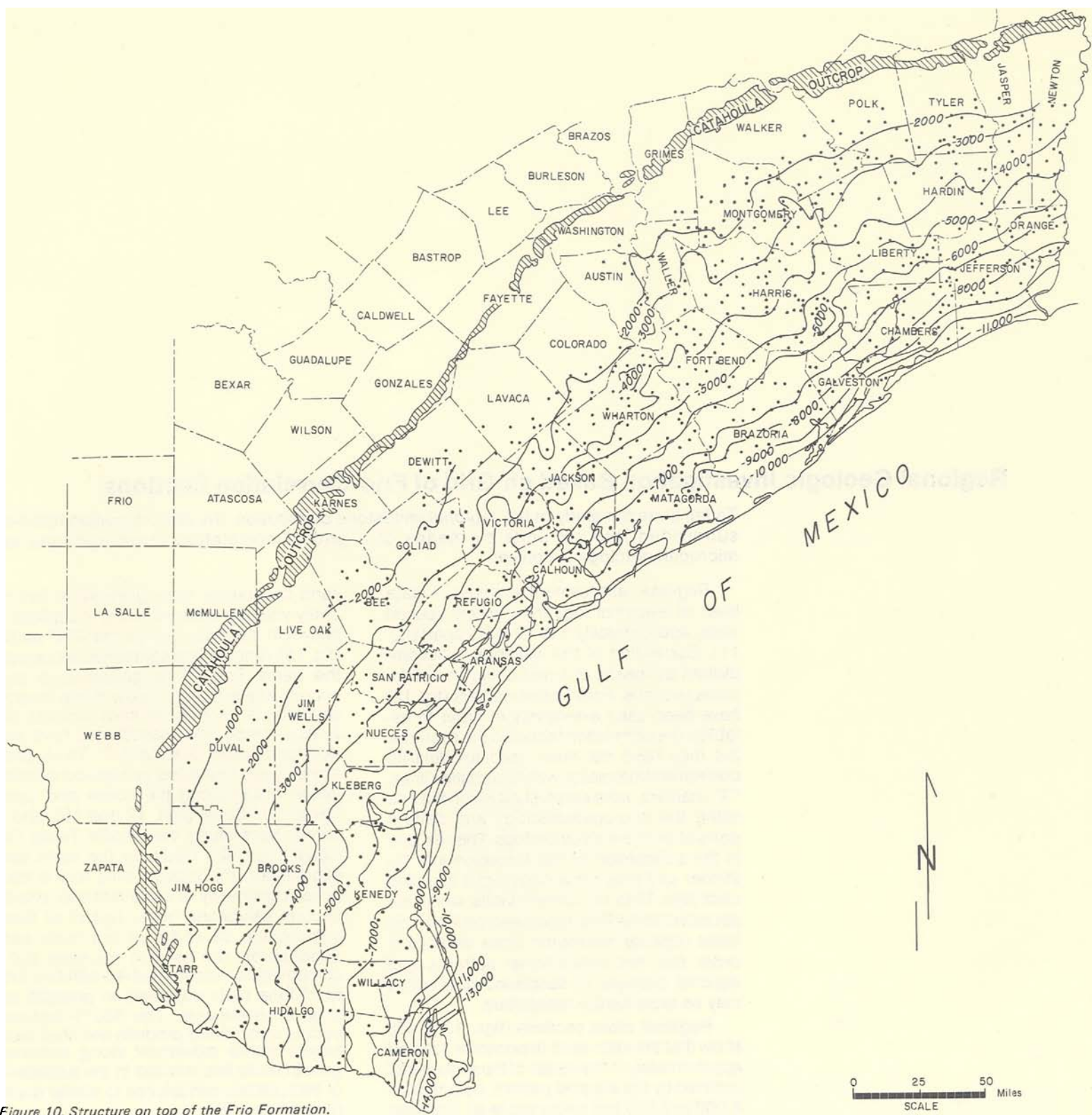
Figure 10. Structure on top of the Frio Formation.
