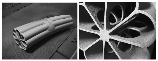
Fig. 3a & 3b. Portion of an A356 structurally optimized and complexly-shaped tube with extensive internal reinforcing features. Investment cast from 3D printed patterns.
