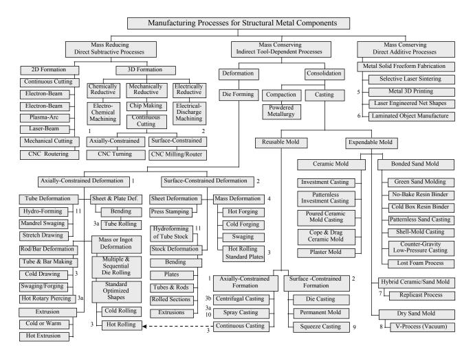
1. Axially-Constrained Formation or Deformation Processes are those that create products with axial or rotational motion. Processes that extrude or roll material through dies or molds generate products that are both axially constrained and constant in cross section. Subractive turning processes create axially-constrained products, but these may vary significantly in cross section.
