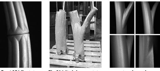
Fig. 7a. A356 Prototype 7b. 316 Stainless prototypes, as cast and powder coated.
