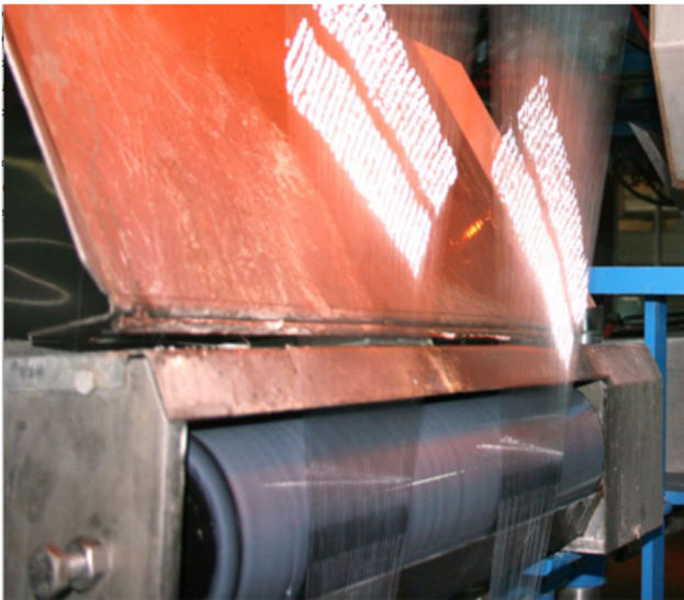
Fig. 2. Close up picture of a sizing applicator in glass fibre production.
