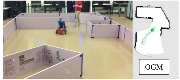
Fig. 3. An example of a mobile robot moving around to map the walls and obstacles of an experimental environment [10].
