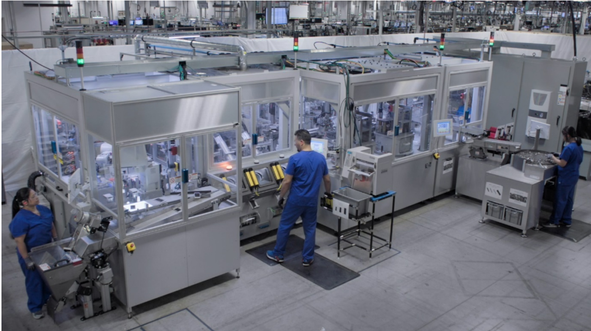
Figure 3: ‘Apple introduces Daisy, a new robot that disassembles iPhone to recover valuable materials’. Source Apple (2018)
