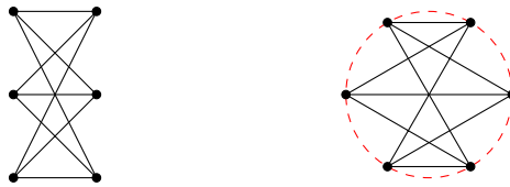
Fig. 2 A rigid placement of the bipartite graph K_{3,3} (left) and flexible placement of same graph with vertices lying on a circle [10, Theorem 14] (right).
