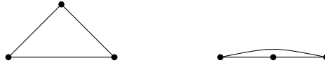
Fig. 4 Two continuously and locally rigid placements of the complete graph K_3 in the Euclidean plane. While the placement on the left is infinitesimally rigid, the placement on the right is infinitesimally flexible. The last bar of the right framework has been drawn curved so that the reader may view it.
