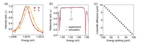
FIG. 10. (a) Energy-resolved emission of the ground-state polariton for horizontal (H) and vertical (V) polarizations, split in energy by around 30  $\mu$ eV. (b) Transfer matrix calculations (red) and experimental reflectivity of the sample. The lower polariton mode (marked by an arrow) is offset by 10 meV below the center of the stop band. (c) Transfer matrix calculations showing the linewidth difference versus the energy splitting. The linewidth difference is 10% of the energy splitting.
