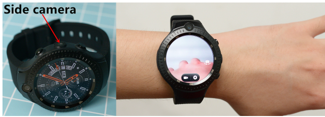
Figure 1. There are smartwatches (e.g., Zeblaze Thor 4 Dual shown here) with a built-in side camera. This can observe the back of hand area and can be leveraged to recognize hand poses and gestures.
