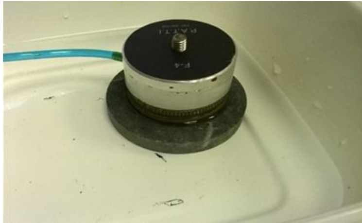
Figure 8: PATTI test, substrate and pull off stub submerged in water and other test assembly
