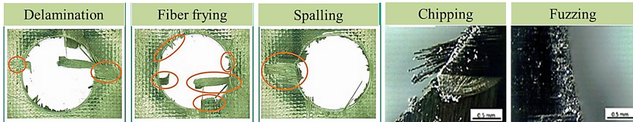
Figure 2: Drilling induced hole damage in FRPs [17]
