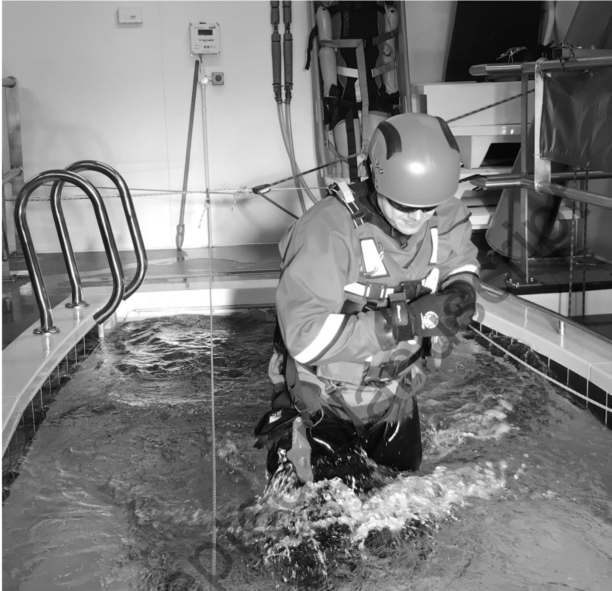
Figure 2. An example of a participant pulling the 10 kg load into the flow of the water during the ‘Warm’ simulation.
