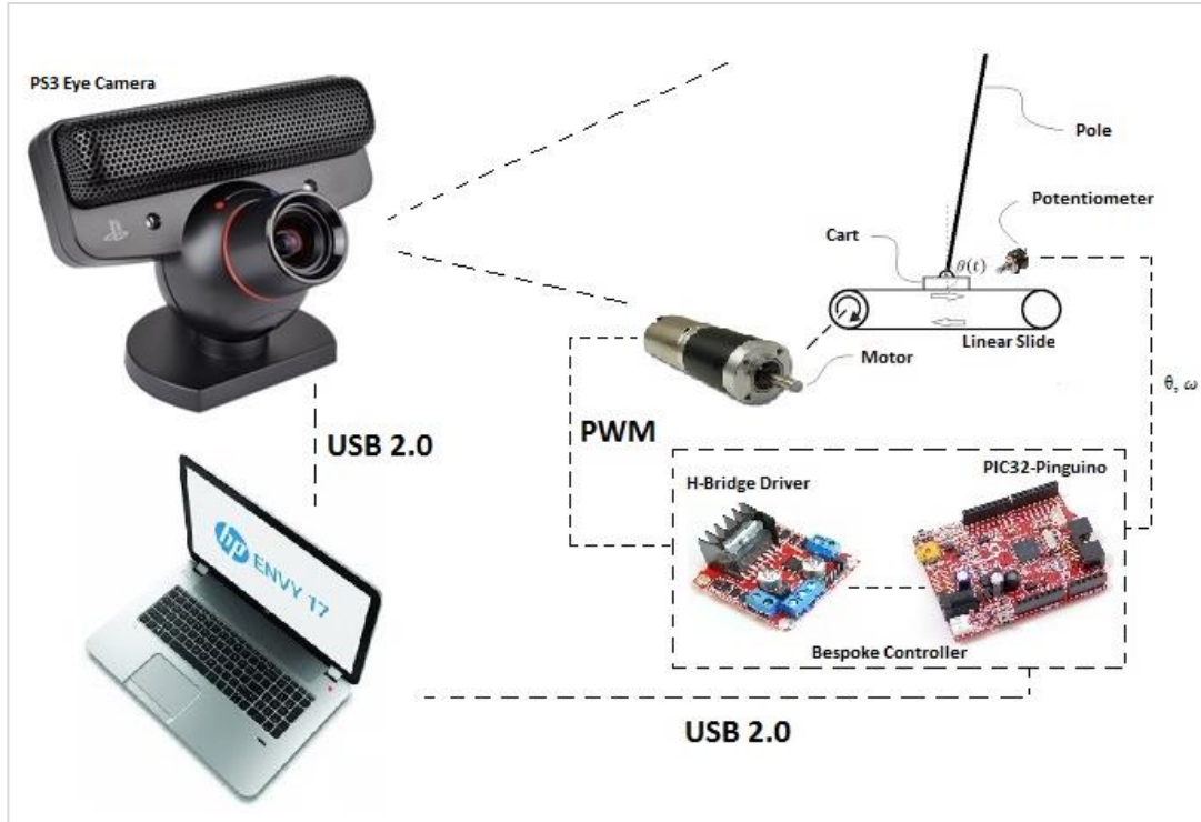
Figure.1.2 – An Overview of the Closed-Loop Cart Inverted Pendulum System.
