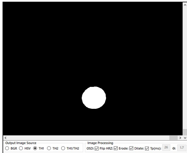
Figure.5.4 – Segmented Image of the Cart Marker.
