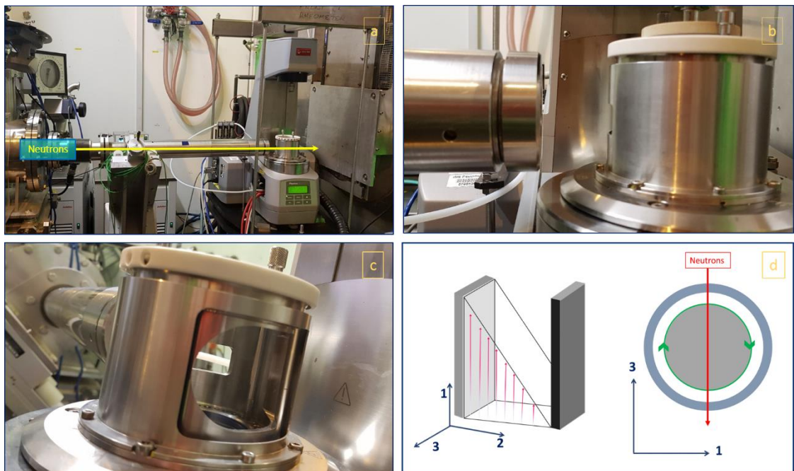
Figure 3-13 Rheo-SANS setup on beamline SANS2D. (a) MCR 501 rheometer mounted in front of SANS2D. (b) and (c) showing close ups of measuring cell. (d) A schematic scattering planes inside the Couette cell, where 1-, 2-, and 3-directions are the coordinate indices representing the flow velocity ( v ), velocity gradient ( \Delta v ) and vorticity ( \omega ) directions, respectively.
