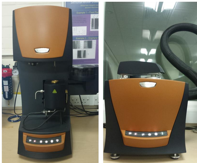
Figure 3-2 (left) TA Discovery TGA and (right) TA Discovery DSC.
