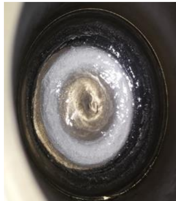
Figure 4-19 A photo of the Couette after the application of the shear ramps at 37°C on F127 20%.
