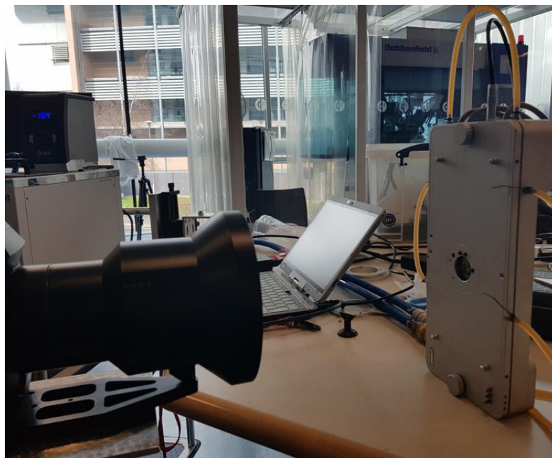
Figure 3-19 FLIR X6540SC IR Thermal Camera with the Linkam shear cell prior to measurement.
