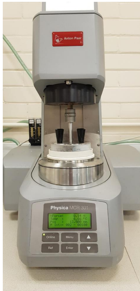
Figure 3-6 Anton-Paar Physica MCR 301 with CC27 and C- PTD200 in use the sample cover.
