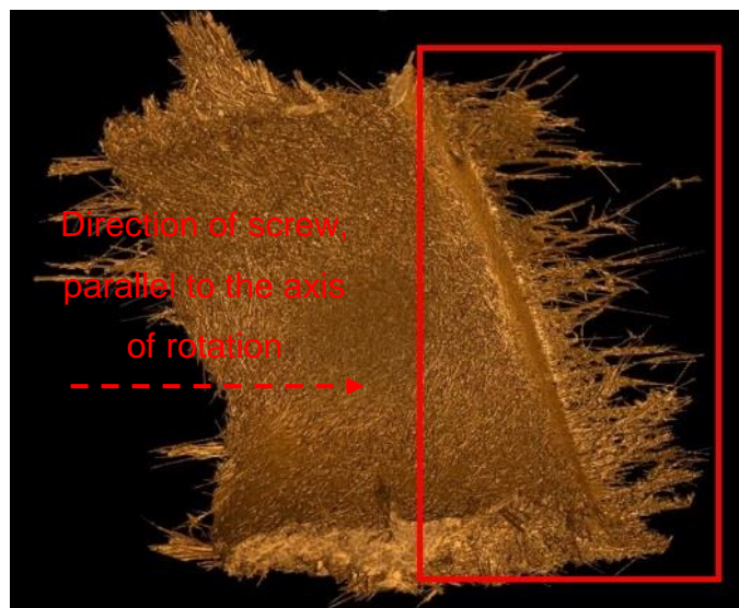
Figure 6.20 - \mu -CT evidence of pellet and screw flight interaction along injection moulding screw
