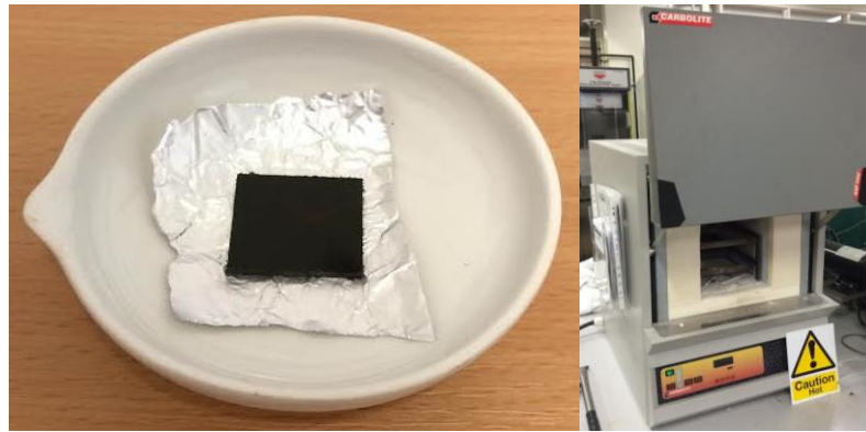
Figure 3.13. - Example of isolated sample placed in ceramic dish (left) and furnace (right).
