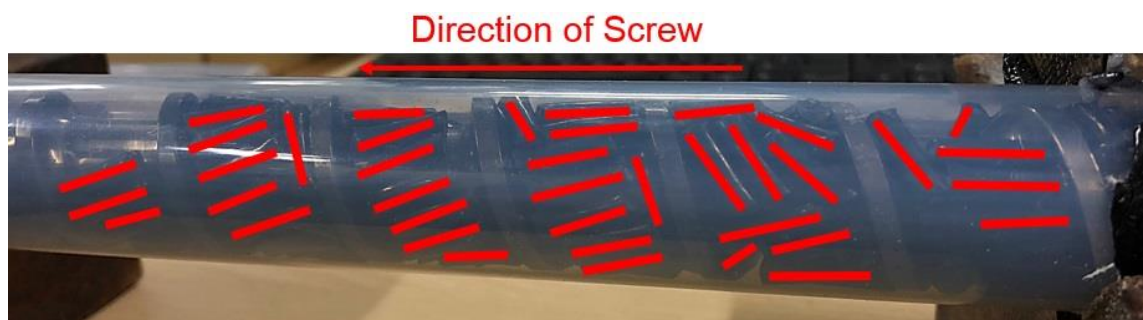
Figure 6.15. – Overlaid lines showcasing example of pellets inclination along an injection moulding screw
