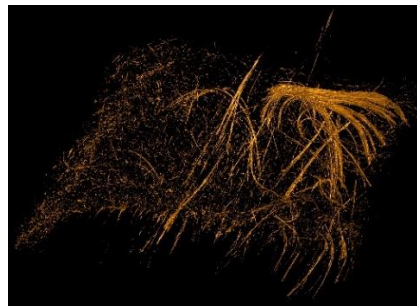
Figure 8.2. - Example of a frayed fibre clusters along the injection moulding process
