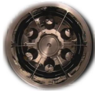
Figure 15: Inside view of the six-segmented cell fluid bed dryer. [4]
