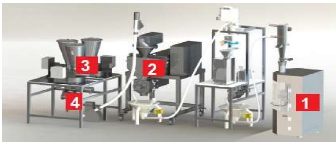
FIGURE 3 - SCHEMATIC FIGURE OF FULL LINE CONFIGURATION – 1. TABLETING MACHINE; 2. ROLLER COMPACTOR; 3. POWDER LOSS IN WEIGHT FEEDERS; 4. CONTINUOUS MIXER (ADAPTED BY (53))
