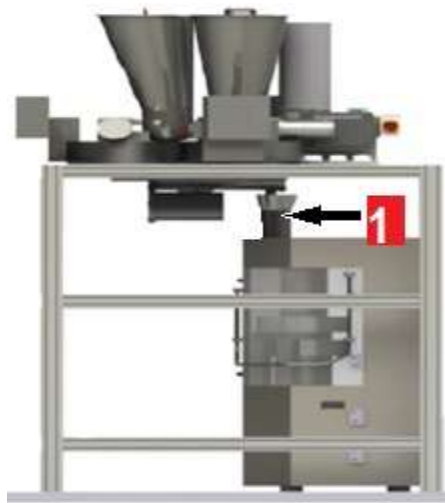
FIGURE 5 - THE DIRECT COMPRESSION CONTINUOUS MANUFACTURING SET-UP USED IN THE EXPERIMENTS. NUMBER 1 LOCATES THE POSITION OF THE NIR SPECTROMETER (ADAPTED FROM (41))
