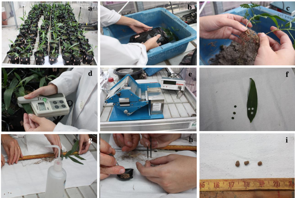
Figure 2.5: Data collection. (a) Experimental set-up at the end of the 20-week experimental period; (b, c) Removal of plants from the pots; (d) Measurement of chlorophyll relative content with SPAD-502; (e) Leaf Area Meter; (f) Removal of phyllode discs for photosynthetic pigments content determination; (g) Measurement of plant components; (h) Removal of root nodules; (i) Examples of root nodules.
