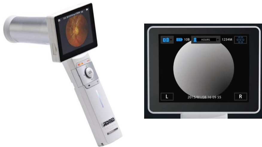
Figure 3.5 Left side: Horus Scope from JedMed. Right-side: Ez Horus Scope observation fundus screen [36]
