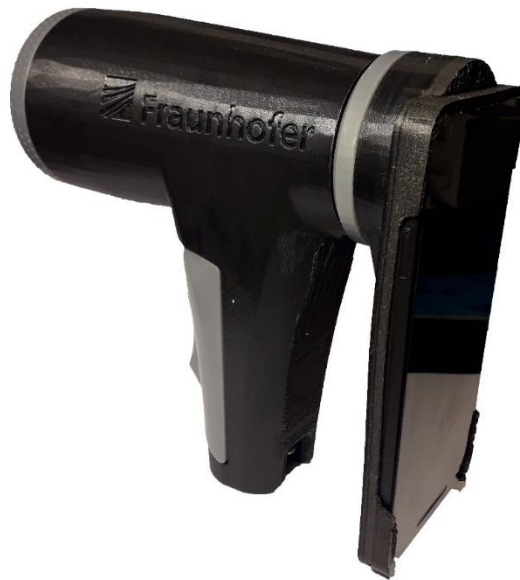
Figure 2.181 Assembled EyeFundusScope prototype
