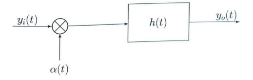
Figure 3.1: Block Diagram of Compressive Receiver Model
