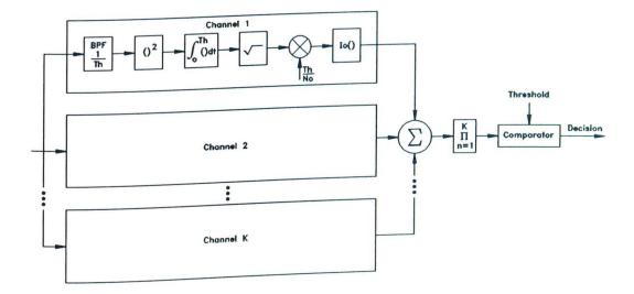
Figure 1.2: Optimal Channelized Detector
