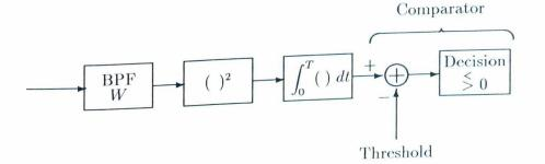
Figure 1.1: Wideband Energy Detector
