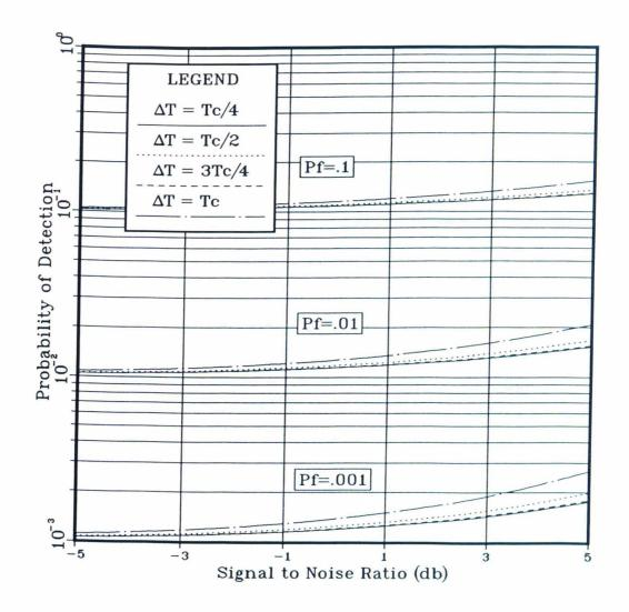
Figure 3.6: Performance of Locally Optimal Detector Compared with Time-Multiplexed Detector, White-Noise Case
