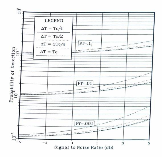
Figure 3.7: Performance of Locally Optimal Detector Compared with Time-Multiplexed Detector, Bandpass Noise Case
