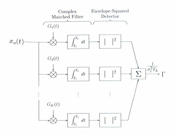
Figure 3.2: Locally Optimal Single-Epoch Detector
