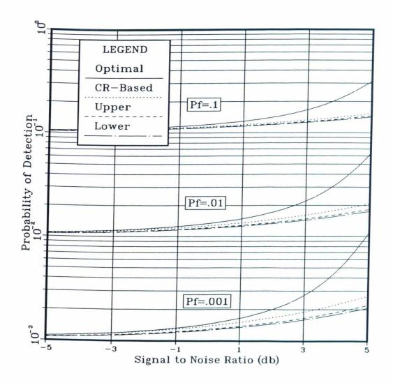
Figure 3.5: Performance of Locally Optimal, Compressive Receiver-Based Detector versus Optimal Detector Based on Direct Observations
