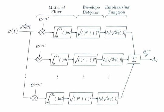
Figure 2.1: Block Diagram of Single-Epoch Likelihood Function
