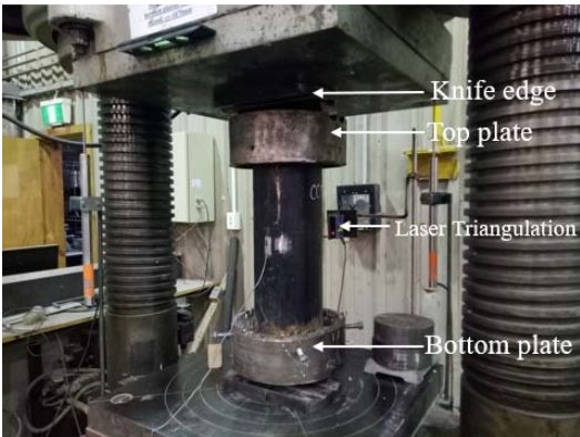
(b) Under eccentric compression
