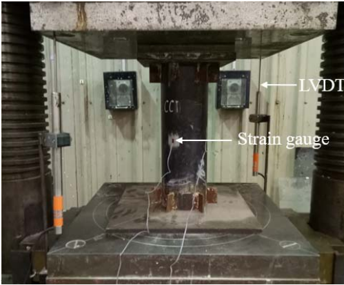
(a) Under axial compression
