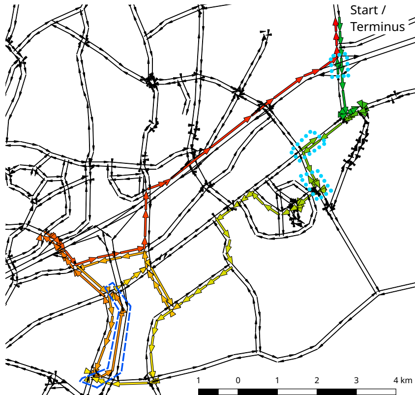
Fig. 2. Example for a circuitous minibus route produced by the evolutionary minibus network design process without penalties for circuitry. Arrows denote the direction of the links, not the stops served. The minibus route starts on the dark green links. The colour of the traversed links changes via yellow to red on the terminus link. In the areas marked in blue the line overlaps itself, i.e. it runs multiple times on the same links.
