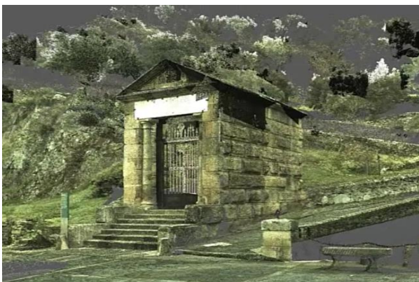
Figure 10: An example of a point cloud. Roman Temple dedicated to the builder Julio Caio Lácer.
