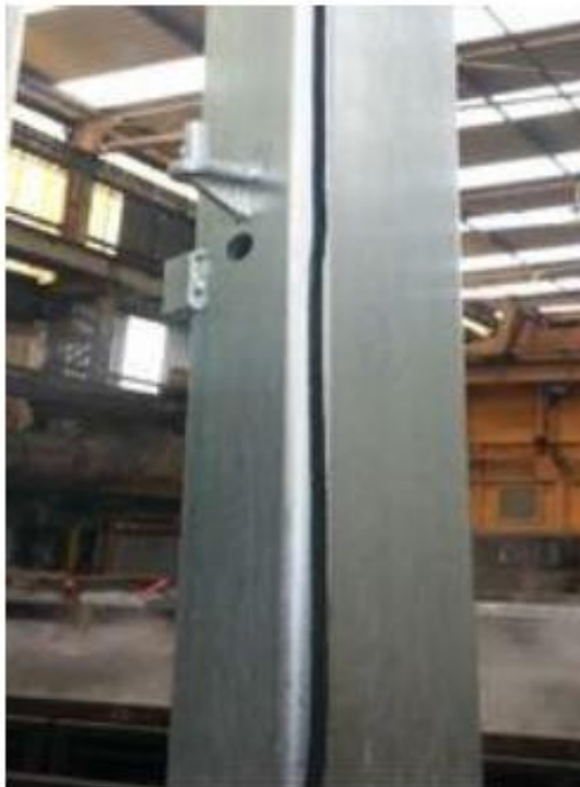
Figure 12 Cracking in a cold formed steel section that has initiated from one end due to the high levels of residual stresses existing in the cold formed section at the corners.
