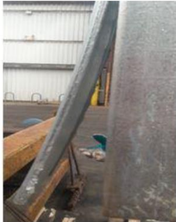
Figure 12 Cracking in a cold formed steel section that has initiated from one end due to the high levels of residual stresses existing in the cold formed section at the corners.
