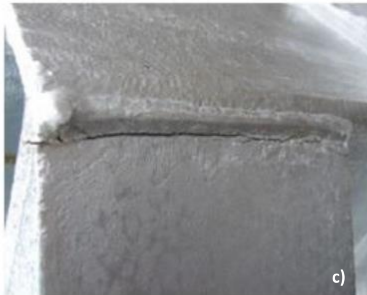
Figure 8 The complex fabrication shown in a) has square box sections b) where several welds are coincident at the highly constrained corners. The interplay among geometric stress concentrations, hardness gradients and residual stresses can very easily either initiate micro-cracks that extend during galvanizing, or initiate LMAC in the galvanizing bath
