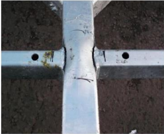
Figure 11 Inadequate venting provision has led to bulging of the main member in the thermally weakened zone where the cross-members were welded to it, causing cracking.
