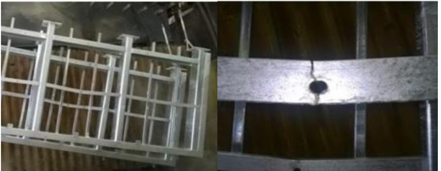
Figure 10 Significant distortion has occurred in the highly constrained smaller cross-members in this steel fabrication, and the off-centre hole has led to an additional localisation of stress, causing cracking to occur during galvanizing.
