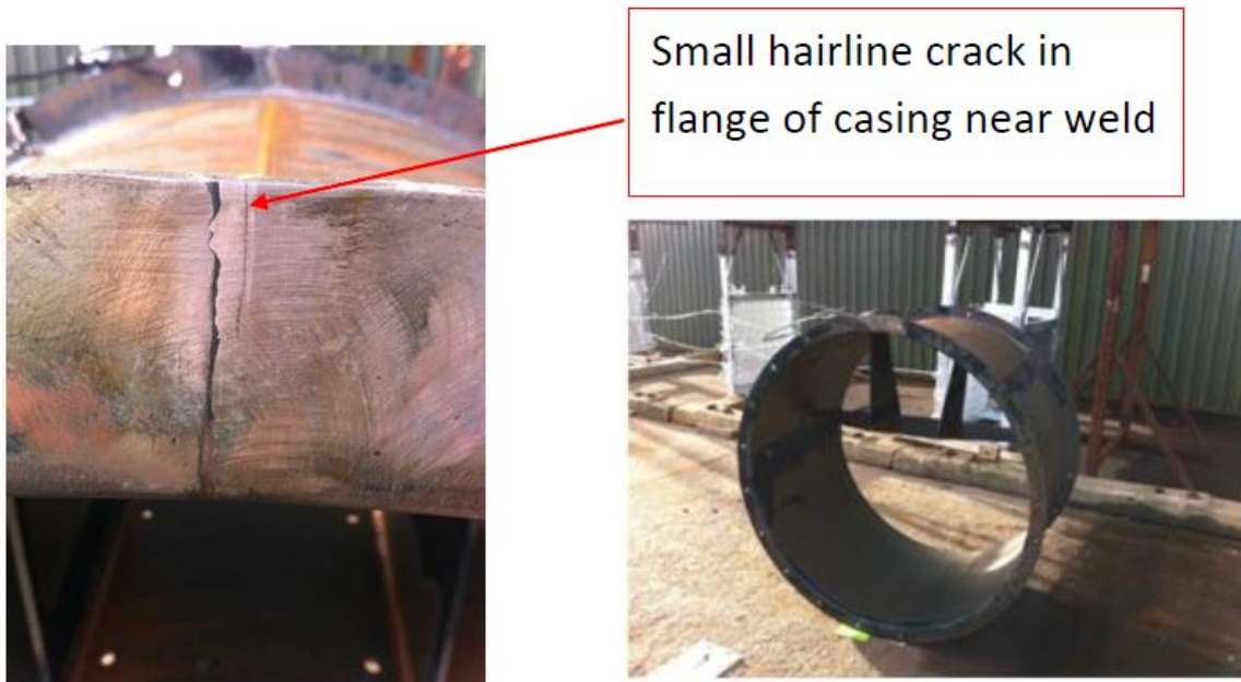
Figure 2 Weld run around an insert that was too close to an existing fabrication-induced region of plasticity/residual stress.
