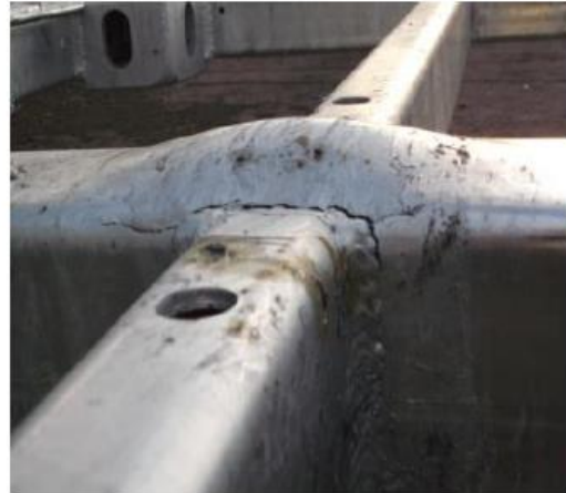
Figure 11 Inadequate venting provision has led to bulging of the main member in the thermally weakened zone where the cross-members were welded to it, causing cracking.
