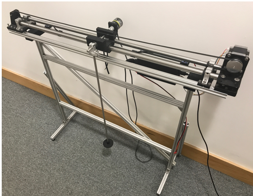
Fig. 3. Pendulum system mounted on its aluminum profile stand. This provides a convenient and elegant means of support and allows the pendulum to rotate freely and avoid collisions.
