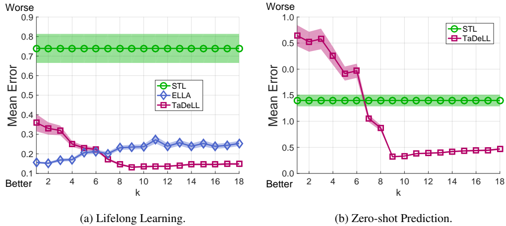
Figure 26: Performance of TaDeLL and ELLA as the dictionary size k is varied for lifelong learning and zero-shot learning. Performance of the single task learner is provided for comparison. In the lifelong learning setting, both TaDeLL and ELLA demonstrate positive transfer that converges to the performance of the single task learner as k is increased. We see that, for this problem, TaDeLL prefers a slightly larger value of k .
