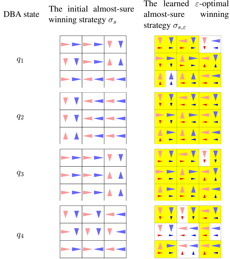
Figure 19: Illustration of the initial almost-sure winning strategy \sigma_s (the middle column) and the learned \varepsilon -optimal almost-sure winning system strategy \sigma_{s,\varepsilon} (the right column). From top to bottom, the four figures in each column show the system strategy with DBA state q_1 to q_4 . In each figure, the pink and blue triangles point to the transition directions at each block when the light is on and off respectively. In the right column, big triangles represent actions with probability (1 - p_{\varepsilon_1}) , and small triangles represent actions with probability p_{\varepsilon_1} . Triangles with yellow background are \varepsilon -optimal over all almost-sure winning system strategies.
