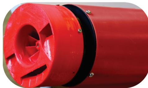
Figure 1. The modular pump-jet thruster for ASV operations in extremely shallow water.
