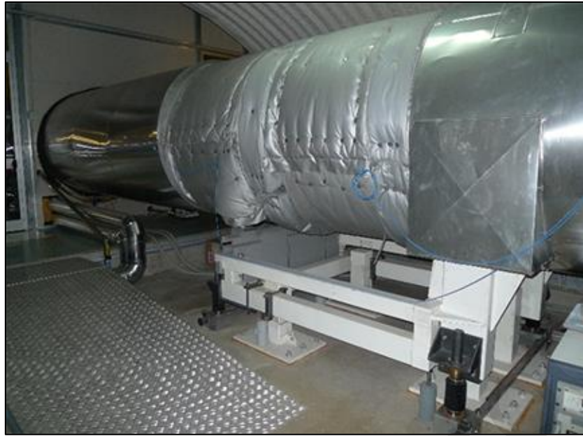
Figure 10. End Building-Tunnel link module. Special tube support with micrometric mechanical realignment system.
