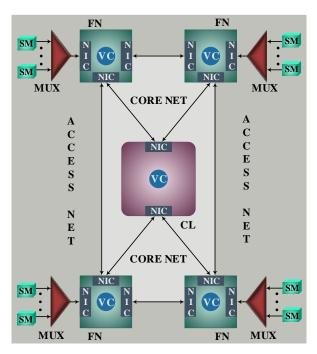
**Figure 1.** A sketch of the proposed SmartFog technological platform. Arrowed paths indicate data links. SM: = Smart-Meter; MUX: = Multiplexer; FN: = Fog Node; CL: = Cloud; VC: = Virtual Clone; NIC: = Network Interface Card.
