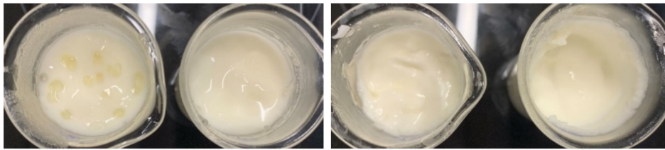
Figure 2. Left: Emulsion after 4 days: left: emulsion with 7% w/w whey protein isolate (WPI) solution; right: emulsion with 8% w/w WPI solution; oil content 73% w/w . Right: Emulsion after 4 days: left: emulsion with 7% w/w sodium caseinate solution; right: emulsion with 8% w/w sodium caseinate solution; oil content 73% w/w .
